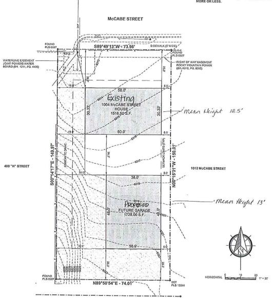
PROPERTY BOUNDARY LINES EXISTING EASEMENTS SETBACK LIMITS ZONING: R-2 (LOW DENSITY RESIDENTIAL) EXISTING FENCE 000 EXISTING OVERHEAD POWER W/POLE AND GUY SETBACKS: FRONT = 20' REAR = 20' SIDES = 10'/6' 0 EXISTING WATER MAIN WITH FIRE HYDRANT M EXISTING TELEPHONE PEDESTAL ----- 6320 -----
